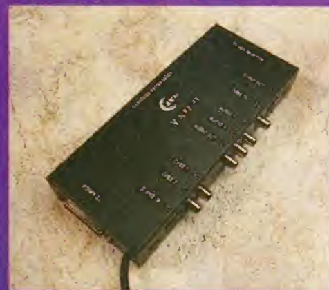
The G-Lock is fully software controlled and handles both Y/C and composite signals.
